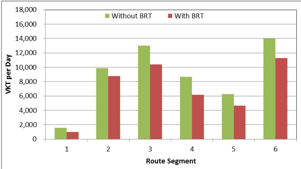
**Exhibit 3-2: Effect of BRT on VKT by Diesel Minibuses by Corridor Segment in 2014**
