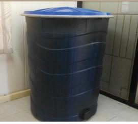
Plastic Storage Silo—adapted for smaller capacity for use by smallholder farmer
