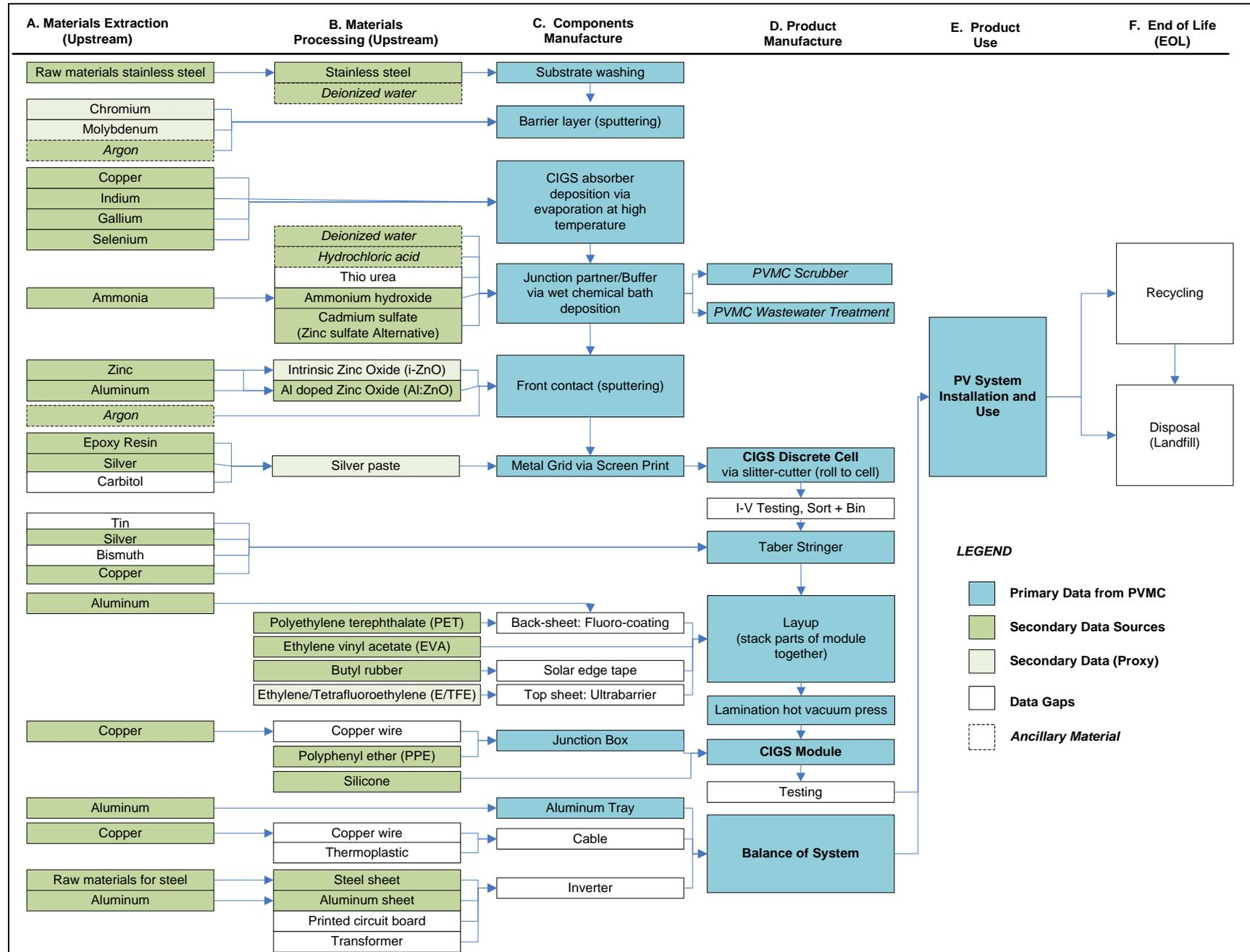
Figure 4. Process Flow Diagram of CIGS Cells Manufactured by PVMC
