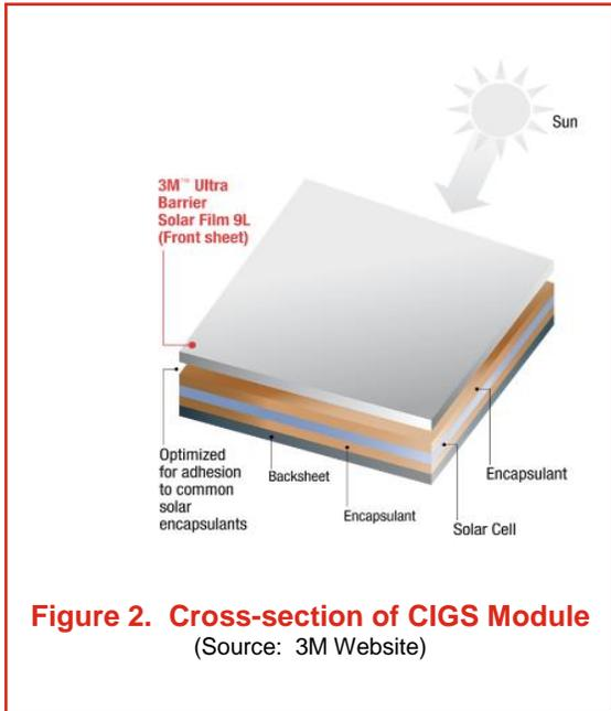
**Figure 2. Cross-section of CIGS Module**
