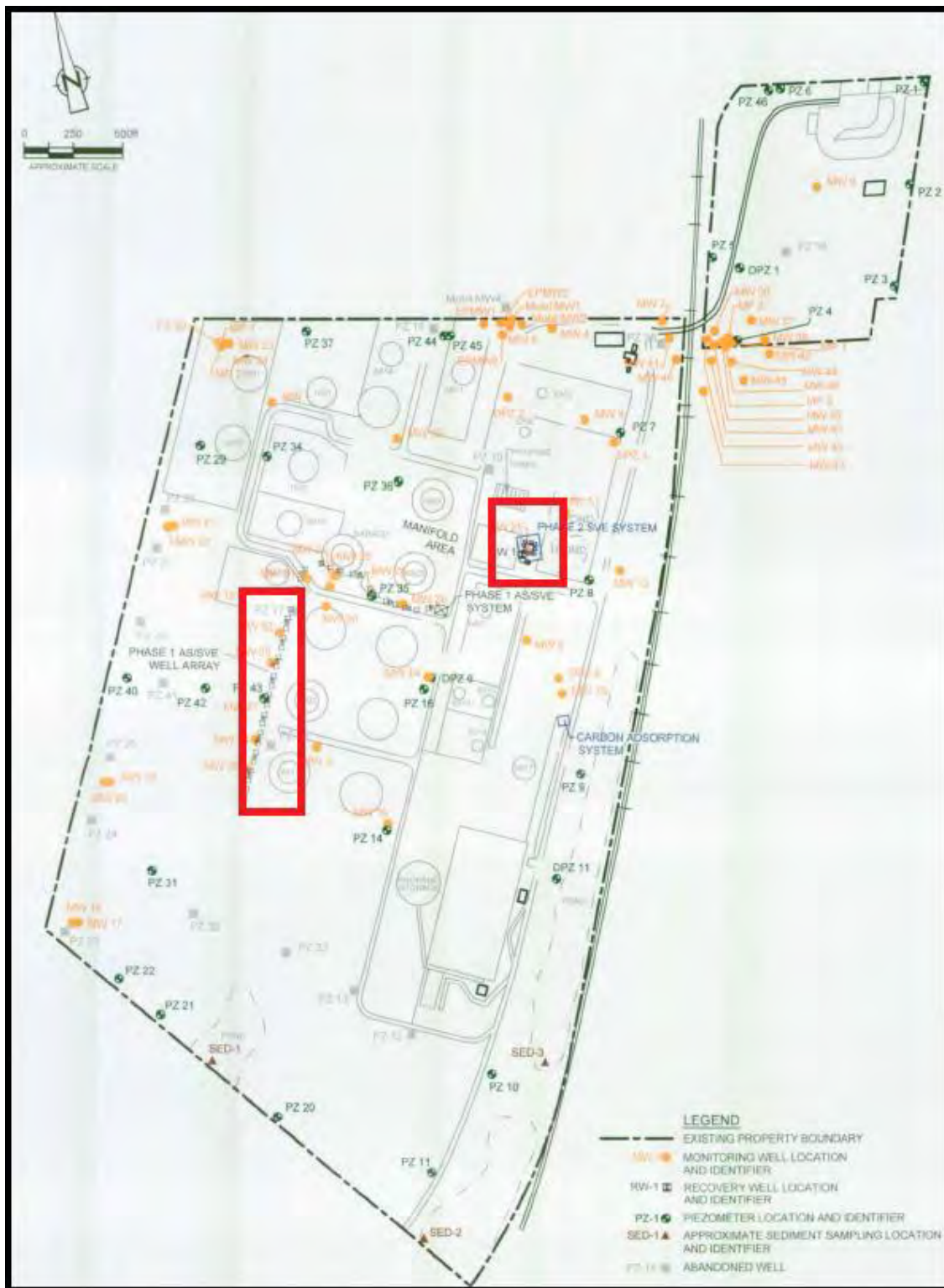
Figure 2.4. Areas at Phillips Petroleum where air sparging and soil vapor extraction are or have been used to address subsurface petroleum releases. The western area is the original “Phase 1” system, and the smaller eastern area is the “Phase 2” system.
