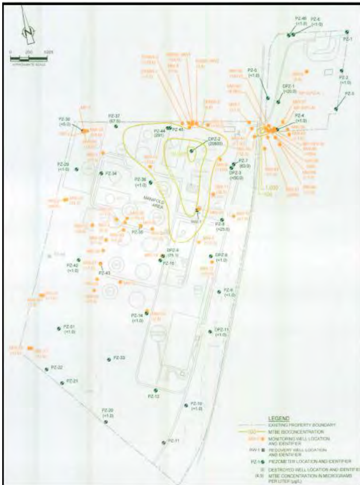
Figure 4.12. Estimated spatial extent of MTBE at the Phillips Petroleum site in May 2016. Note that the lowest concentration contour is 100 µg/L and the injury threshold is 70 µg/L; there are additional wells south of the plume in this figure that exceed 70 µg/L.
