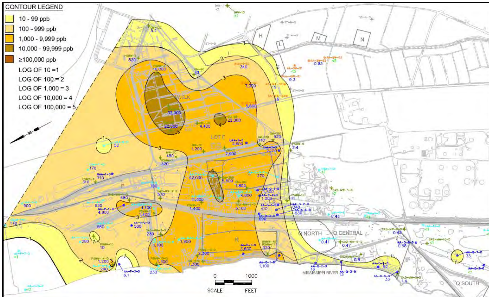
Figure ES.5. Chlorobenzene in the DHU, as depicted in the Sauget Area 2 RI. Note that north is to the left. The injury threshold for chlorobenzene is 100 ppb, which is contour level “2” in this figure.
