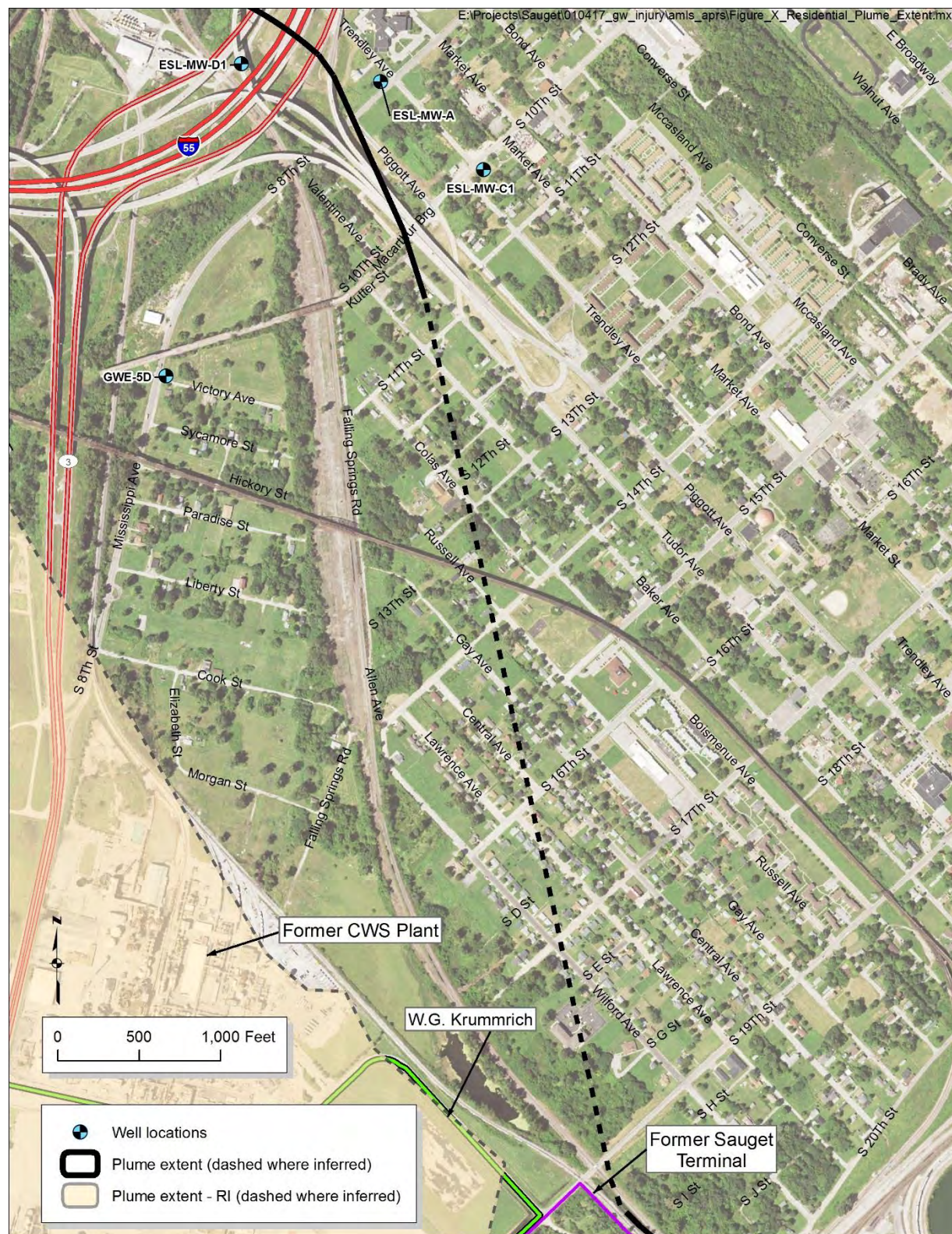
Figure 4.21. Existing groundwater data suggest that benzene and chlorobenzene plumes extend beneath residential areas of East St. Louis. The lack of data from this area is a data gap that the State Trustees intend to address.
