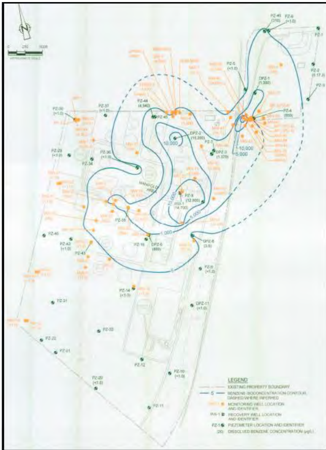
Figure 4.11. Estimated spatial extent of benzene at the Phillips Petroleum site in May 2015. High concentrations at the upgradient property boundaries suggest other potential sources in the area. The dashed lines indicate data gaps.
