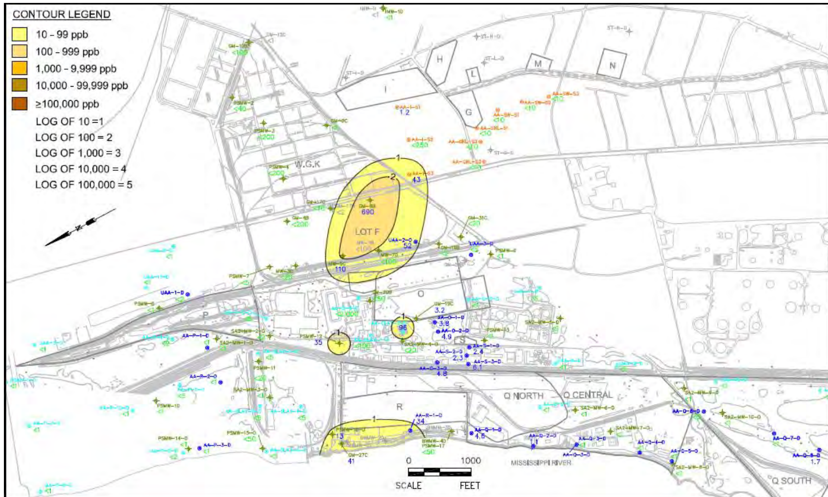
Figure 4.24. Vinyl chloride in the DHU, as depicted in the Sauget Area 2 RI/FS. The MCL and the Class I standard for vinyl chloride is 2 µg/L (ppb). In this figure, the wells near Clayton Chemical all exceed 2 µg/L but are not highlighted because the lowest contour interval is 10 µg/L. Areas where detection limits exceed the MCL include the well line near Site G (10 µg/L), areas under W.G. Krummrich (200 µg/L), and several wells north of the indicated plume extent (5–50 µg/L).
